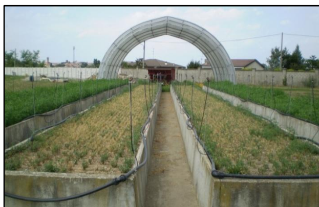
Figure 1. One of CRA-FLC's phenotyping platforms; it includes four environments formed by the combination of two soil types (sandy-loam or silty-clay) by two possible water regimes (applied via microirrigators under a moving shelter)
