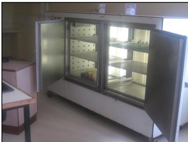
**Figure 3. Insect rearing incubator with controlled temperature and humidity**
