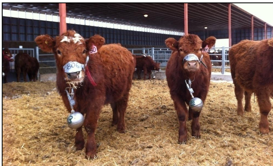
Figure 2. Cattle wearing the methane collection devices
